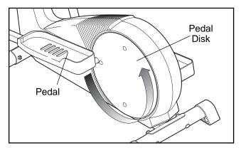
To dismount the elliptical trainer, allow the pedals to come to a complete stop. **CAUTION:** The elliptical trainer does not have a free wheel; the pedals will continue to move until the flywheel stops. When the pedals are stationary, step off the highest pedal first. Then, step off the lowest pedal.
